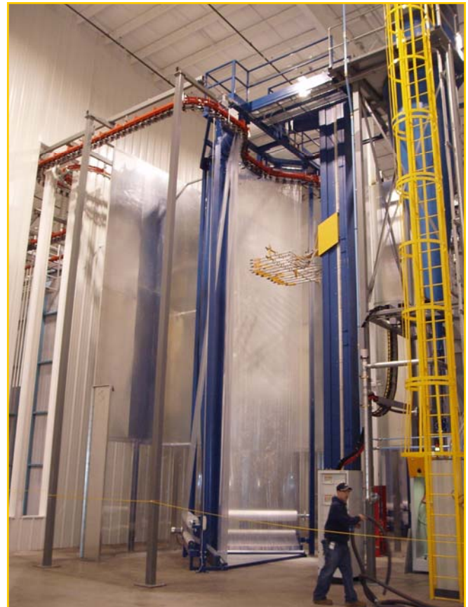
Vertical Powder Coating Booth Designed to Process Aluminum Extrusions with a Maximum Length of 25'-0"
