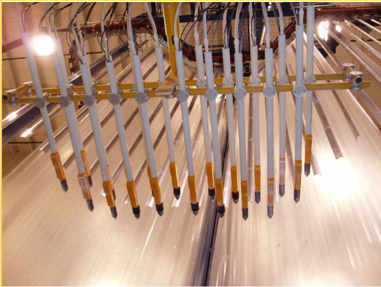
High efficiency powder application equipment mounted on a full stroke reciprocator.
