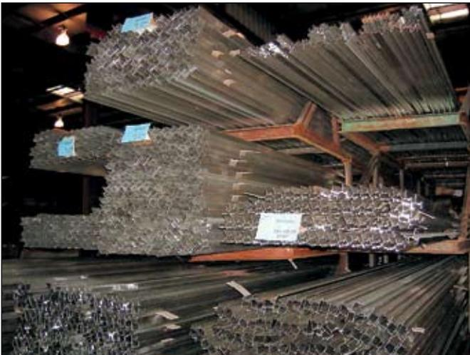
Figure 6. Extrusions stacked and color labeled for finishing on the wet or powder lines.
