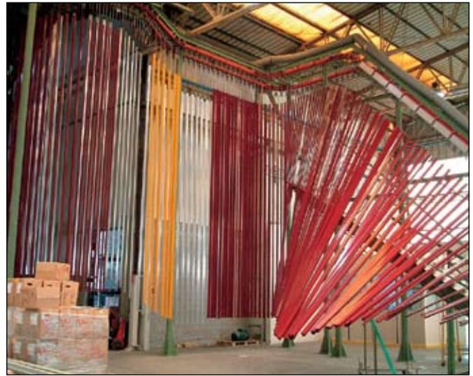
Figure 7. Small lots run with different colors (six profiles in yellow painted between regular run of red profiles) on the vertical powder line at Extruders with no loss of production.
