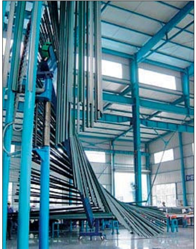
Figure 4. Unloading zone on the vertical powder line.
