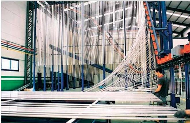
Figure 2. Aluminum extrusions being loaded onto a vertical powder line.
